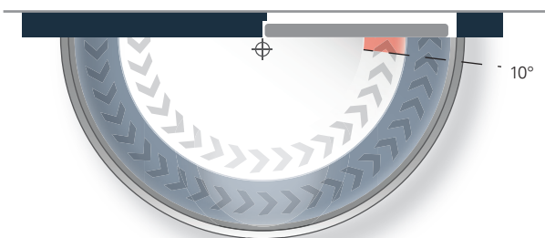
Closing force diagram ECO Newton TS-14, hinge side
